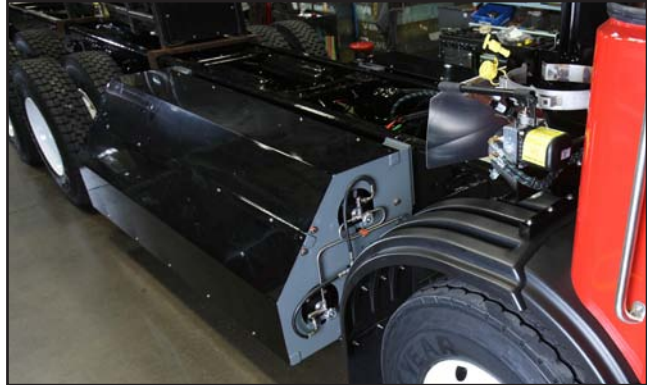
Side frame rail mounted CNG tank on ACX
