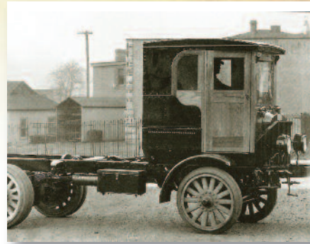
Type XXVII from the 1920's, "Engine under the seat design"
