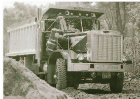
Early 70's S64B Dump Truck with "super size" radiator
